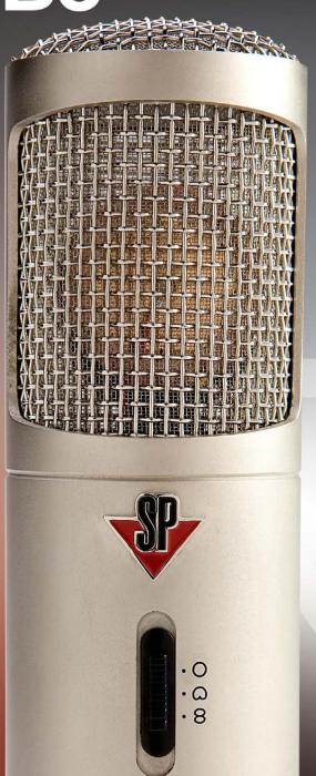
The Studio Projects® B3 is a large diaphragm condensor microphone with 3 recording patterns and dual 1" 3 micron gold sputtered capsules manufactured using our pressure gradient technology. Equipped with 6dB/octave High Pass Filter (@150Hz) and a -10dB Pad, it is not only versatile but has an exceptional linear response and world class sound.
